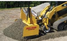
**Dual Dozer** Capable of 3D, GPS, Laser, Sonic and Slope Sensing, Dual Dozer can achieve any sub-grading goals. Expect reduced labor, time and material overages.
