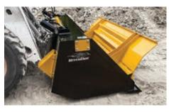
Patent Pending Push-Off Bucket Increase dump cycle times with this patent pending product all while minimizing wear and tear on equipment by no longer 'shaking' sticky materials.
